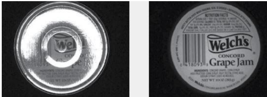
Figure 5 (a): Reflections from of a sealed cap illuminated by ambient light and a white LED light source. This results in specular glare that renders the cap unreadable. After installing polarizing film over the light source and either using a polarizing filter on a standard monochrome camera or, by using a polarizing camera, will greatly reduce any specular reflections (Image courtesy MidOpt).
