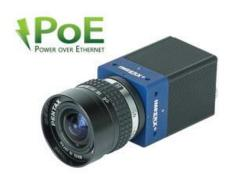
The cameras support resolutions from 3 megapixels to 12 megapixels in optical formats ranging from 1/1.8" to 1.1" with 8, 10, and 12-bit outputs. The Sony Pregius sensors have global shutters with 3.45-micron and 4.5-micron square pixels delivering high sensitivity and wide dynamic range up to 80dB. Exceptional thermal design allows 16 second or longer exposure times without the need for forced air cooling.
