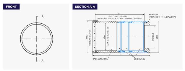
Base lens tube cavity length is 36 mm. Other lengths can be achieved by using one or more extenders.
