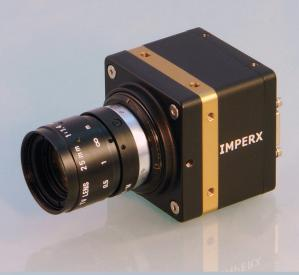
IMPERX ICL-B0610 is an advanced progressive scan, fully programmable CCD camera designed for imaging applications that require high quality images, powerful features and flexibility. The camera is small, light weight, and built around the TRUESENSE Imaging KAI-0340 7.4 micron interline transfer CCD image sensor with a 1/3" optical format.
