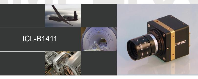
IMPERX ICL-B1411 is an advanced progressive scan, fully programmable CCD camera designed for imaging applications that require high quality images, powerful features and flexibility. The camera is small, light weight, and built around Sony's ICX-267 4.6 micron Interline Transfer CCD image sensor with a 1/2" optical format.
