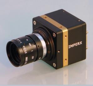
IMPERX ICL-B1610 is an advanced progressive scan, fully programmable CCD camera designed for imaging applications that require high quality images, powerful features and flexibility. The camera is small, light weight, and built around SONY's ICX-274 4.4 micron interline transfer CCD image sensor with a 1.1/8" optical format.
