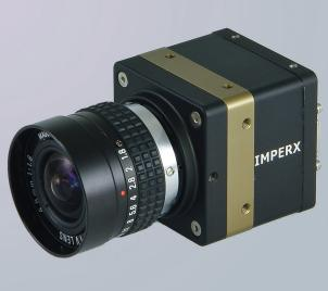
IMPERX ICL-B1920 is an advanced progressive scan, fully programmable CCD camera designed for imaging applications that require high quality images, powerful features and flexibility. The camera is small, light weight, and built around TRUESENSE Imaging's KAI-2093 7.4 micron interline transfer CCD image sensor with a 1" optical format.
