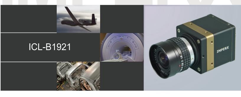
IMPERX ICL-B1921 is an advanced progressive scan, fully programmable CCD camera designed for imaging applications that require high quality images, powerful features and flexibility. The camera is small, light weight, and built around TRUESENSE Imaging's KAI-02150 5.5 micron interline transfer CCD image sensor with a 2/3" optical format.
