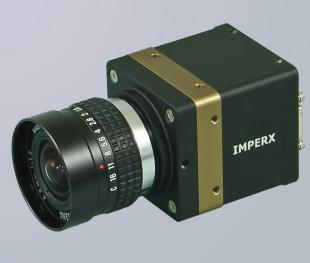
IMPERX ICL-B2510 is an advanced progressive scan, fully programmable CCD camera designed for imaging applications that require high quality images, powerful features and flexibility. The camera is small, light weight, and built around SONY's ICX-655, 3.45 micron interline transfer CCD image sensor with a 2/3" optical format.
