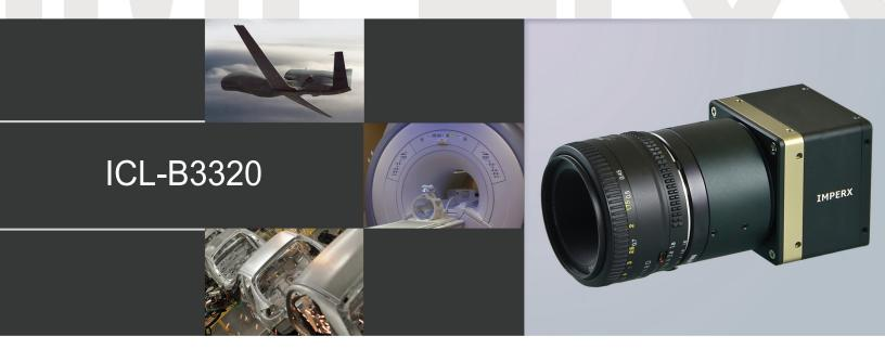
IMPERX ICL-B3320 is an advanced progressive scan, fully programmable CCD camera designed for imaging applications that require high quality images, powerful features and flexibility. The camera is small, light weight, and built around TRUESENSE Imaging's KAI-08050 5.5 micron interline transfer CCD image sensor with a 1.3" optical format.
