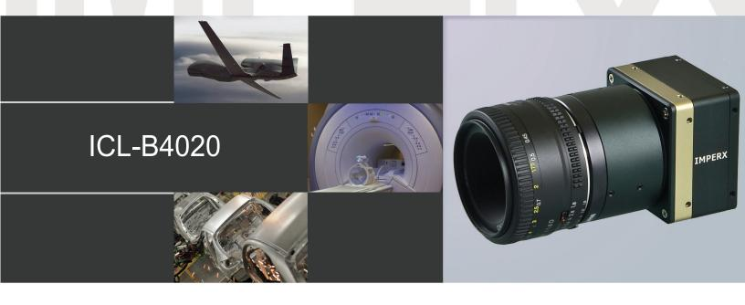
IMPERX ICL-B4020 is an advanced progressive scan, fully programmable CCD camera designed for imaging applications that require high quality images, powerful features and flexibility. The camera is small, light weight, and built around TRUESENSE Imaging's KAI-11002 9 micron interline transfer CCD image sensor with a 43.3 mm optical format.
