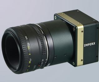
IMPERX ICL-B4820 is an advanced progressive scan, fully programmable CCD camera designed for imaging applications that require high quality images, powerful features and flexibility. The camera is small, light weight, and built around TRUESENSE Imaging's KAI-16000 7.4 micron interline transfer CCD image sensor with a 43.3mm optical format.
