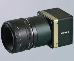
IMPERX ICL-B4821 is an advanced progressive scan, fully programmable CCD camera designed for imaging applications that require high quality images, powerful features and flexibility. The camera is small size, light weight, and built around TRUESENSE Imaging's KAI-16050 5.5 micron interline transfer CCD image sensor with a 32.36mm optical format.
