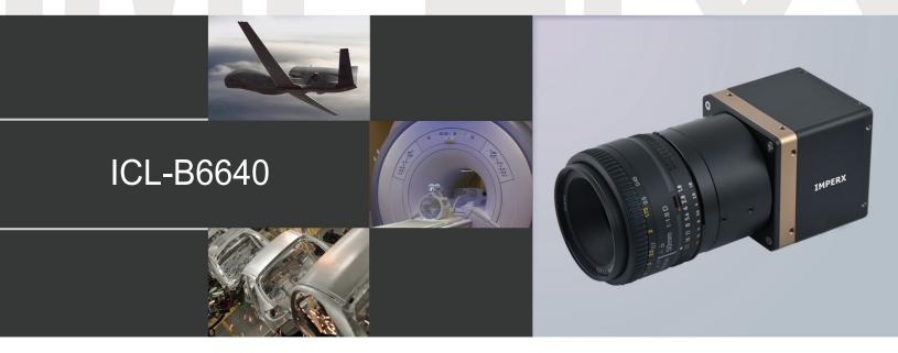
IMPERX ICL-B6640 is an advanced progressive scan, fully programmable CCD camera designed for imaging applications that require high speed, brilliant images, powerful features and flexibility. The camera is small, light weight, and built around the TRUESENSE Imaging KAI-29050, 4-tap, 5.5 micron interline transfer CCD image sensor with a 43.47mm optical format.
