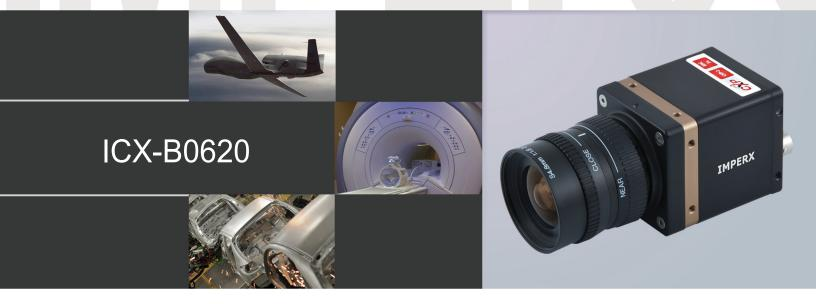
**IMPERX** ICX-B0620 is an advanced progressive scan, fully programmable CCD camera designed for imaging applications that require high guality images, powerful features and flexibility. The camera is small, light weight, and built around the TRUESENSE Imaging KAI-0340 7.4 micron interline transfer CCD image sensor with a 1/3" optical format.
