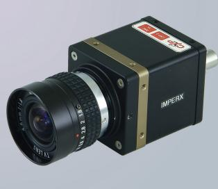
IMPERX ICX-B1410 is an advanced progressive scan, fully programmable CCD camera designed for imaging applications that require high quality images, powerful features and flexibility. The camera is small, light weight, and built around Sony's ICX-285 6.45 micron interline transfer CCD image sensor with a 2/3" optical format.
