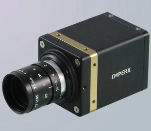
IMPERX IGV-B1410 is an advanced progressive scan, fully programmable CCD camera designed for imaging applications that require high quality images, powerful features and flexibility. The camera is small, weight, and built around SONY's ICX-285 6.45 micron interline transfer CCD image sensor with a 2/3" optical format.
