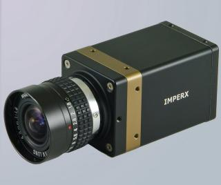
IMPERX IGV-B2320 is an advanced progressive scan, fully programmable CCD camera designed for imaging applications that require high quality images, powerful features and flexibility. The camera is small, light weight, and built around the TRUESENSE Imaging KAI-04050 5.5 micron interline transfer CCD image sensor with a 1" optical format.
