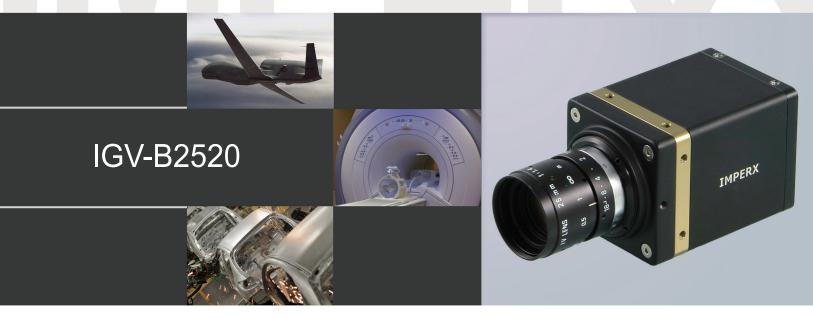
IMPERX IGV-B2520 is an advanced progressive scan, fully programmable CCD camera designed for imaging applications that require high quality images, powerful features and flexibility. The camera is small, light weight, and built around SONY's ICX-625 3.45 micron interline transfer CCD image sensor with a 2/3" optical format.
