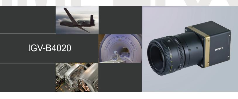
IMPERX IGV-B4020 is an advanced progressive scan, fully programmable CCD camera designed for imaging applications that require high quality images, powerful features and flexibility. The camera is small, light weight, and built around the TRUESENSE Imaging KAI-11002 9 micron interline transfer CCD image sensor with a 43.3 mm optical format.
