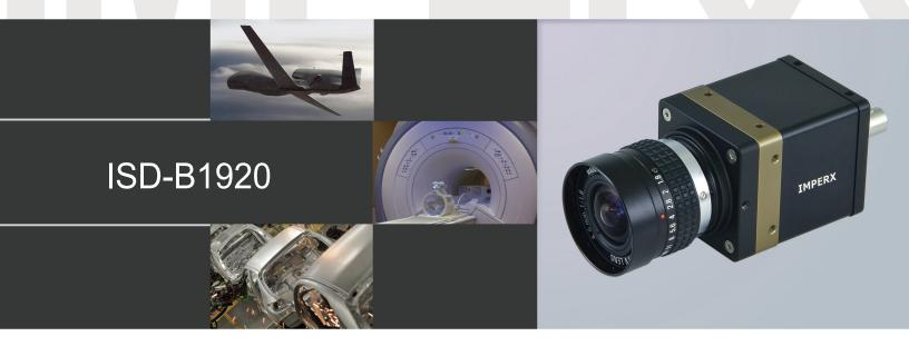
IMPERX ISD-B1920 is an advanced progressive scan, fully programmable CCD camera designed for imaging applications that require high quality images, powerful features and flexibility. The camera is small, light weight, and built around the TRUESENSE Imaging KAI-2093 7.4 micron interline transfer CCD image sensor with a 1" optical format.
